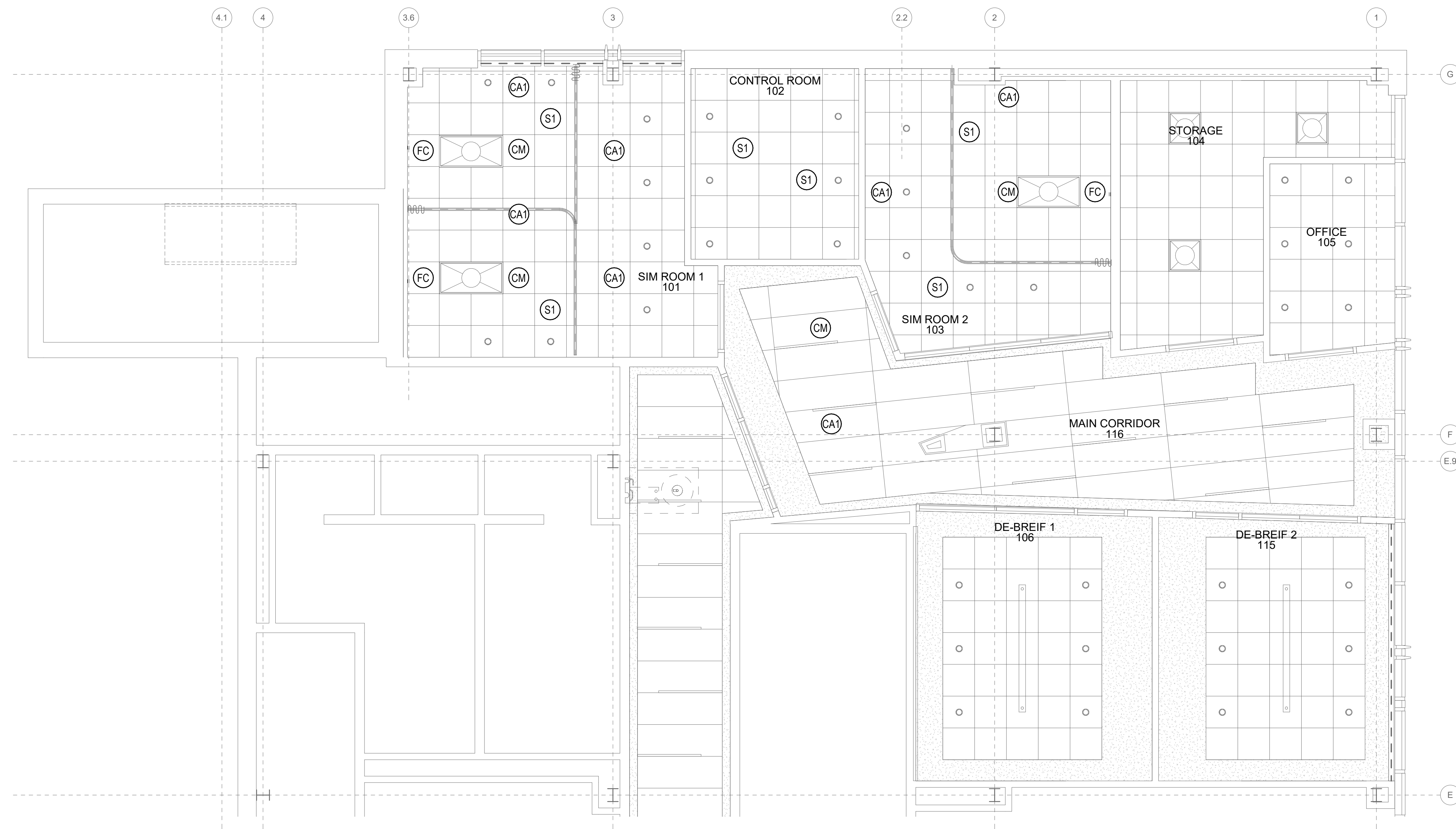
3 AUDIOVISUAL REFLECTING CEILING PLAN - LEVEL 04 1/4" = 1'-0"
